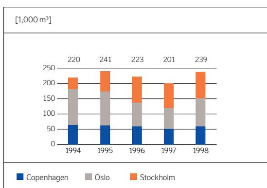
**SAS's development:** Water consumption has increased at all of the main airports and particularly in Oslo (Fornebu). This was due to problems with recirculation of cooling water from the electroplating process to the water reservoir.
