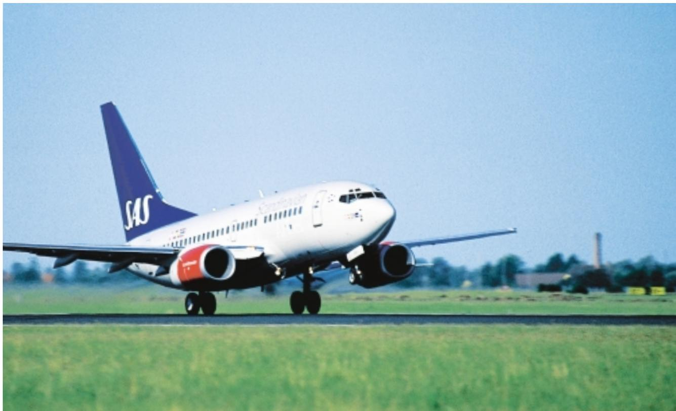
1999 was the first full year with a number of SAS's new Boeing 737s in operation, with DAC engines that dramatically reduce NO<sub>x</sub> emissions.
